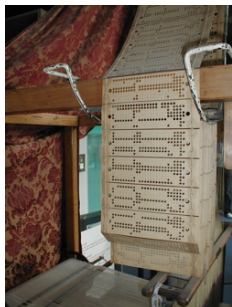
Figure 5: A Jacquard loom using punched card. Figure source-wikipedia
